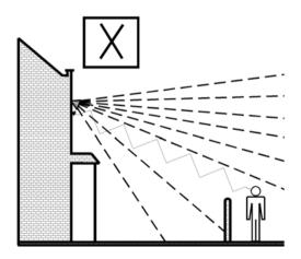
Movement detectors can be useful if they are correctly installed and aimed. Unfortunately, many systems do not allow the detector to be separately aimed from the floodlight.
