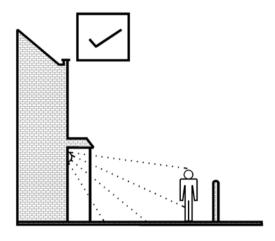
Besides being cheap to run, this type of light is kinder to the environment providing a gentle wash of light with reduced glare. Bulkhead and porch lights cast fewer shadows reducing the hiding places for criminals. These units can be fitted with a movement detector if required. These units are generally mounted lower and are therefore less susceptible to nuisance switching and complaints from neighbours.
