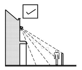
Floodlights and detectors should be aimed to only detect and light people on your property. They should not detect a person or animals walking down the street. If the floodlight is fitted with a timer, this should be adjusted to the minimum to reduce the operation of the light.
