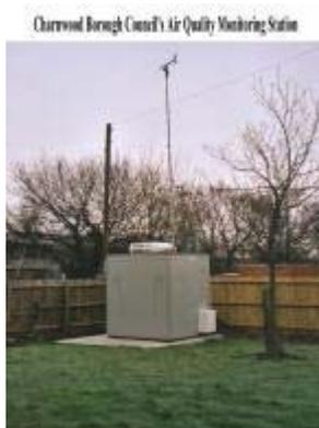
It has a small weather station with a thermometer, wind direction vane and wind speed meter that help to interpret the information the station collects. We periodically place all of our portable monitoring equipment alongside the station to compare the results.
