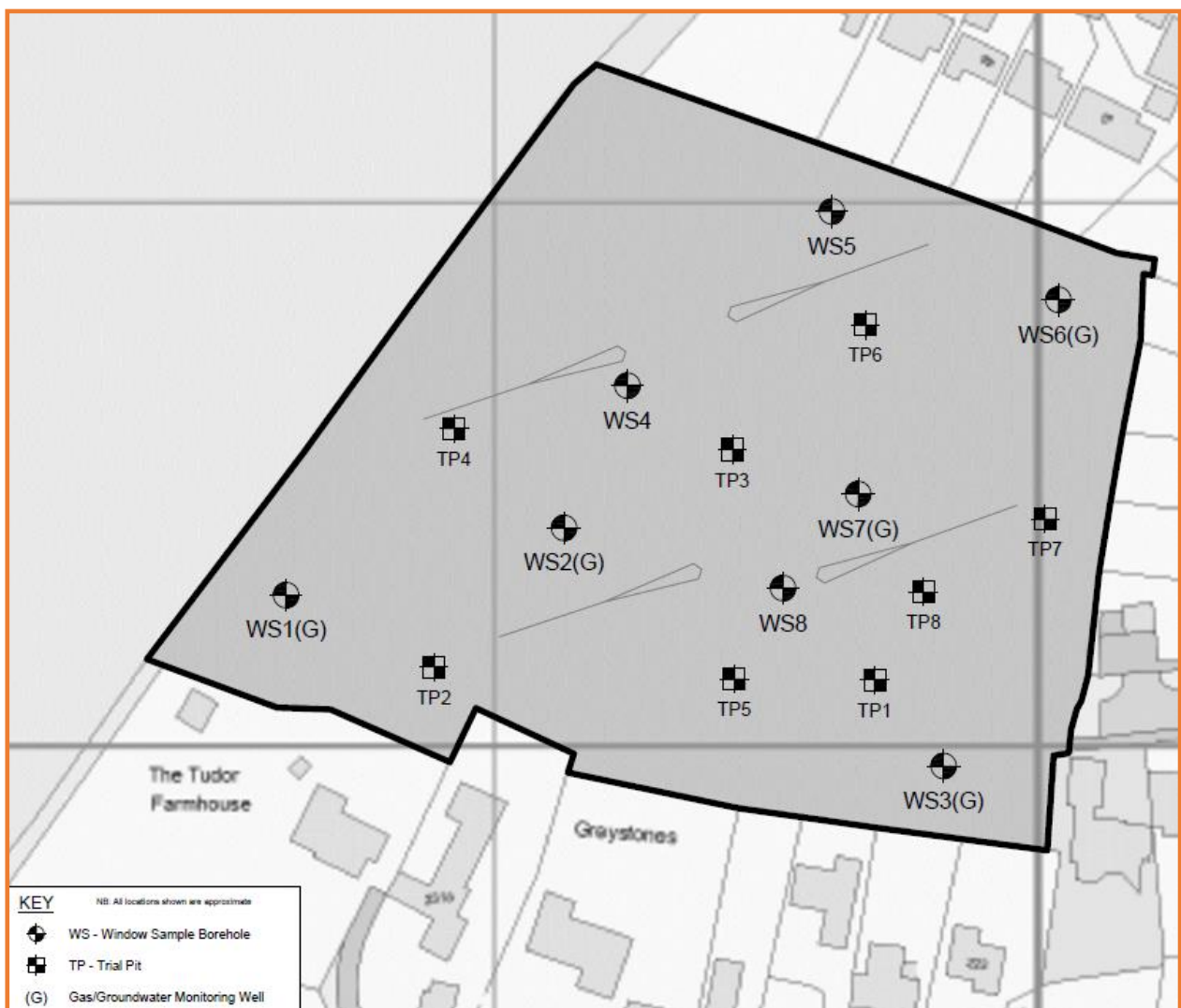
Figure 3: Ground investigation exploratory hole location plan.
