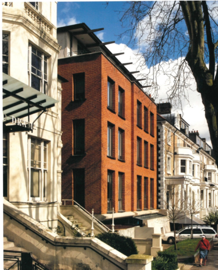
Above: This contemporary building in London contrasts greatly with the surrounding character in terms of detailing and exterior materials however it respects the street scape by way of its scale, mass and height, and it respects the common building line (image source: Historic England/CABE, 2001)
