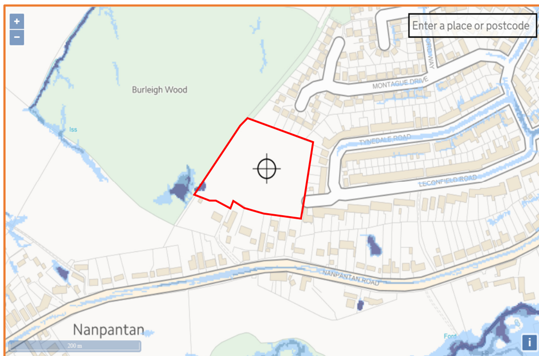
Figure 5 - The pluvial flood risk to the site.
