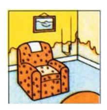
Rising damp will only affect basements and ground floor rooms. It will normally rise no more than 12 to 24 inches above ground level (300mm to 600mm) and usually leaves a 'tide mark' low down on the wall. You may also notice white salts on the affected areas.
