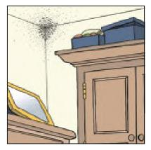
Condensation is caused by water vapour or moisture from inside the dwelling coming into contact with a colder surface, such as a window or wall. The resultant water drops (condensation) may then soak into the wallpaper or paintwork or even plasterwork. In time, the affected damp areas then attract black mould that grows on its surface.
