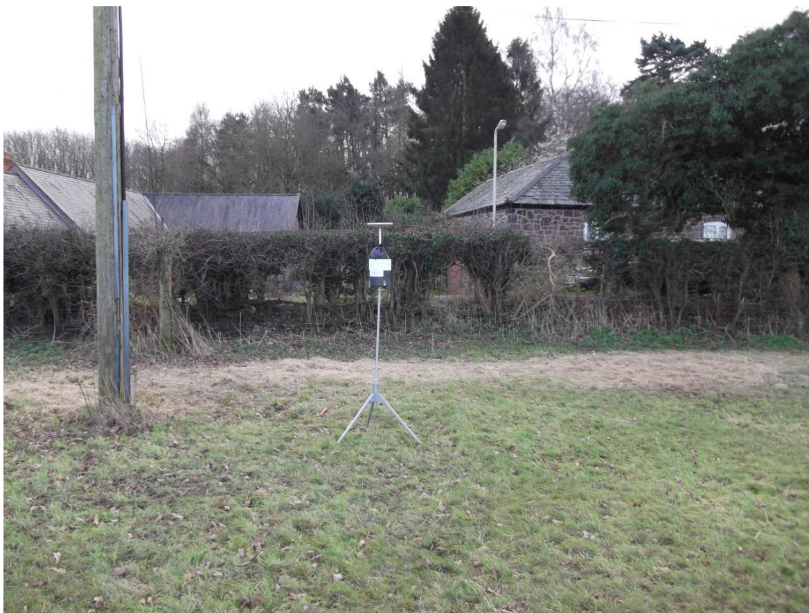
Figure 4: Supplementary dust monitor towards the eastern end of Kinchley Lane (Stn 1A)
