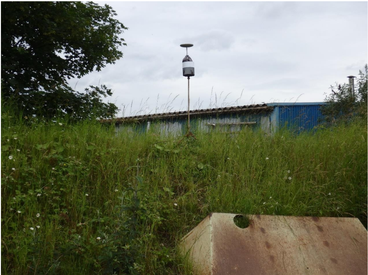
Figure 3: Long-term combined 'Frisbee-type' deposited dust gauge with adhesive directional dust sampler at Railhead (Stn 6A)
